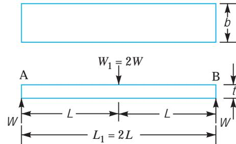
Fig. 23.27. Flat spring (simply supported beam type).
