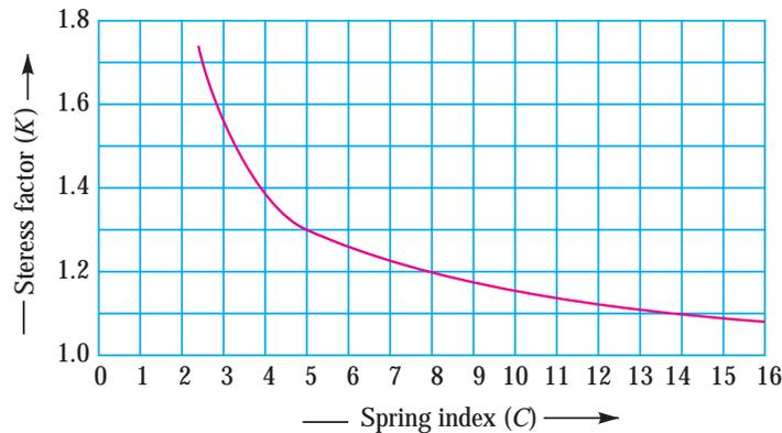
Fig. 23.12. Wahl's stress factor for helical springs.
