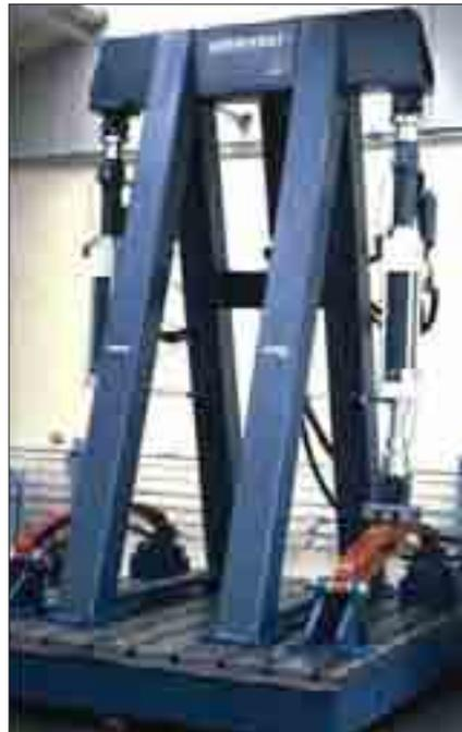
Leaf spring fatigue testing system.
