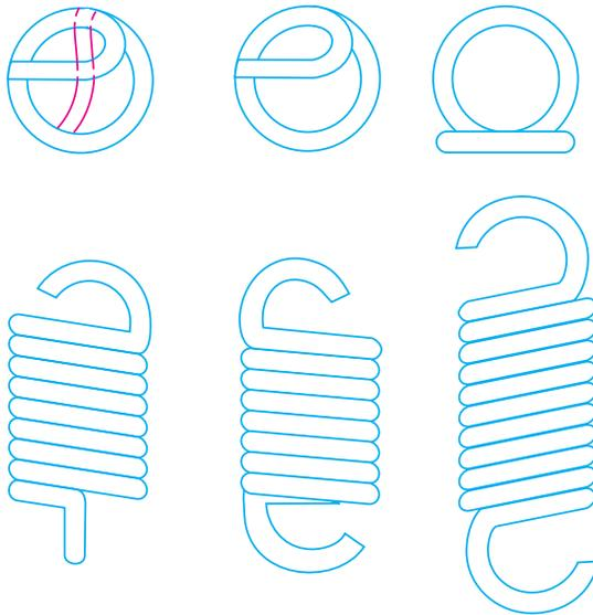
**Fig. 23.8.** End connection for tension helical springs.
