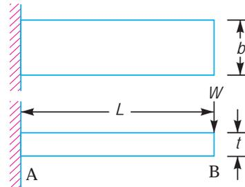
Fig. 23.25. Flat spring (cantilever type).
