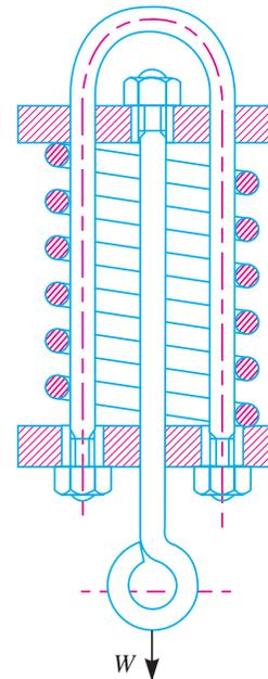
**Fig. 23.9.** Compression spring for carrying tensile load.
