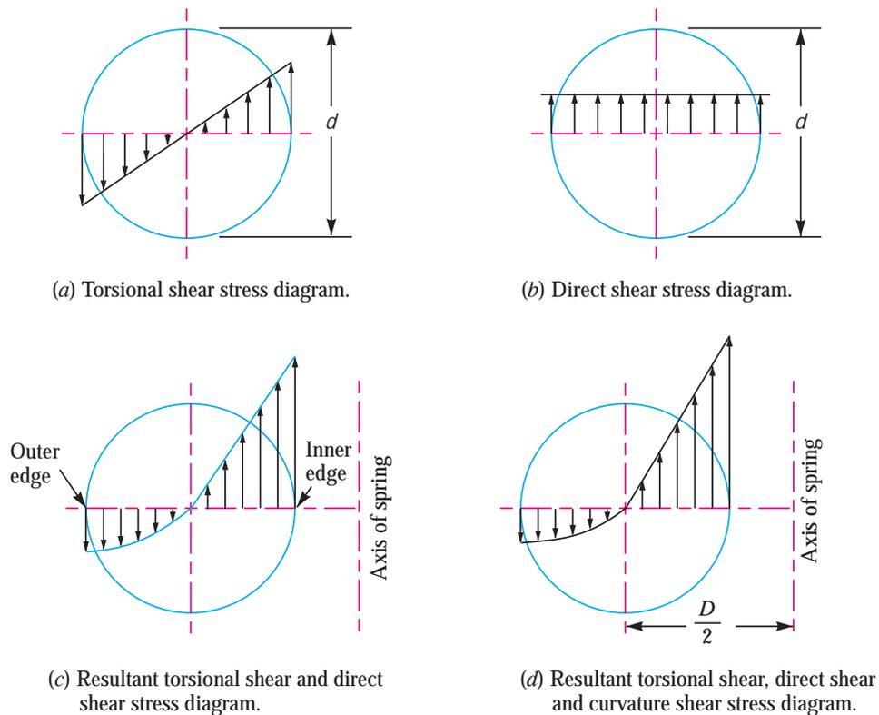
**Fig. 23.11.** Superposition of stresses in a helical spring.
